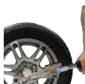
Completion of tightening process with Blue signal.
