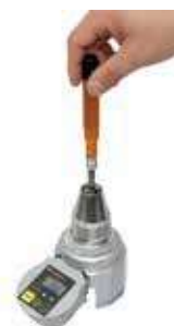
BMRD torque checking with BTGE-G.
