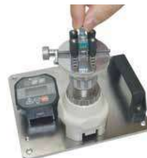
ATGE-G with table attachment and measurement stand
