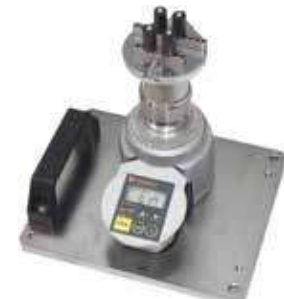
BTGE-G with table attachment and measurement stand
